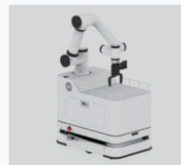
OSH200-C-DIFF-S 底盘+载物箱体+协作机械臂一体化整机（复合型作业机器人） Integrated machine of chassis + cargo box + collaborative robotic arm (composite operation robot)
