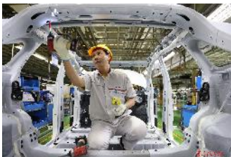
Interior Installation Workstation The robotic arms cannot reach the required operating space
