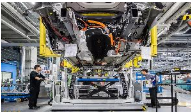
Wiring harness installation station Robotic arms cannot install flexible wiring harnesses.
